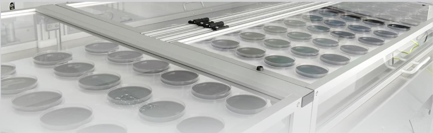
When very high output per hour is required, IQ Designs offers two models of 8-lane filling machines. The IQ-HSL High Speed Petri Dish Filling Machine has 8-lanes and specializes in the filling of 90 mm mono plates up to 12,000 plates per hour. This filling machine is for serious producers that need tens of thousands of plates filled per day cleanly and efficiently.
