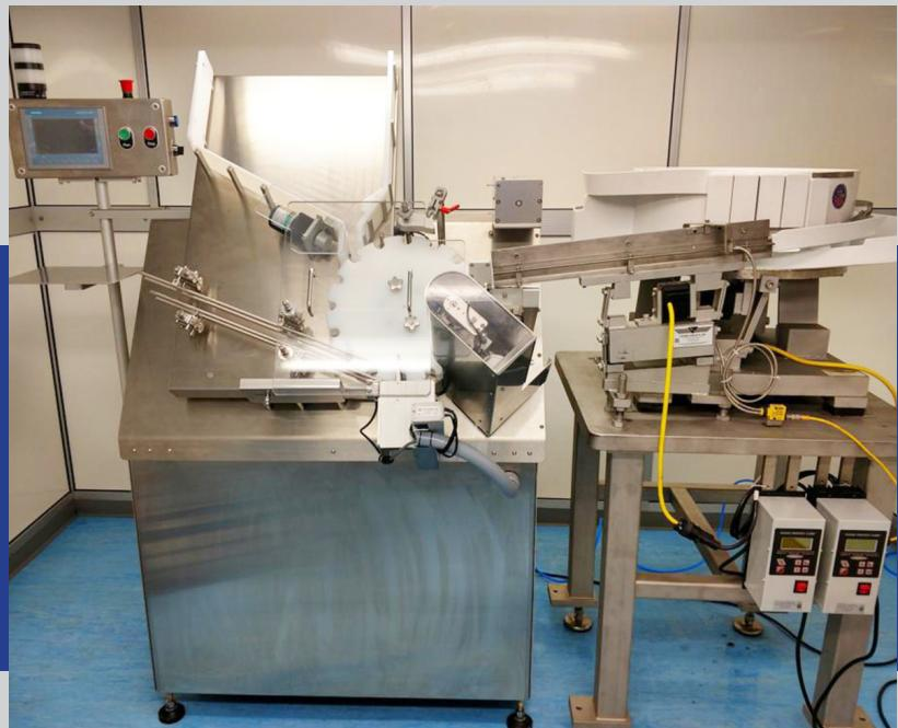
verification) and an output conveyor with accumulation station at the end. It can also be upgraded to print directly on the side of the tube, or label the tube. If you need automated racking, we can automatically place finished tubes into the racks of your choice.
