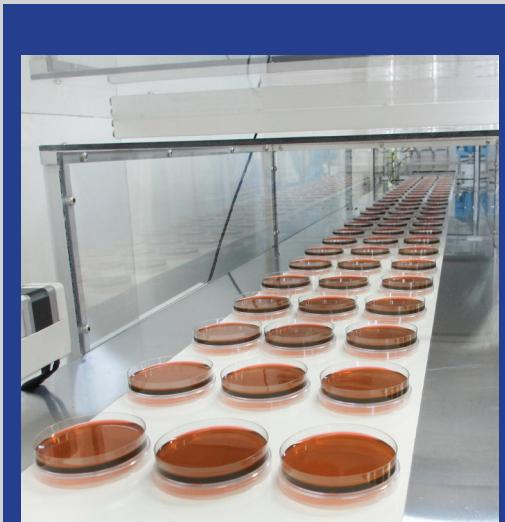
The IQ-M2000 Petri Dish Filling Machine can run multiple dish types. By changing out a few "Change Parts" you can switch from one dish type to another, in less than 10 minutes!
