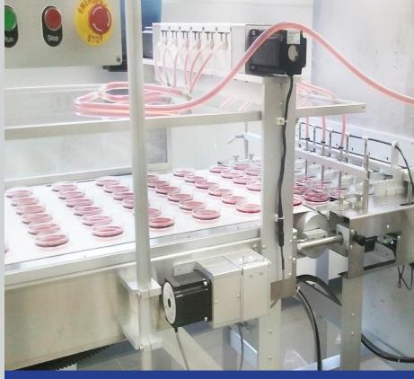
The IQ Designs Petri Dish filling machines feature additive peristaltic pumps as standard equipment.
