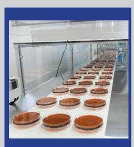
The IQ-M2000 Petri Dish Filling Machine can run multiple dish types. By changing out a few "Change Parts" you can switch from one dish type to another, in less than 10 minutes!
